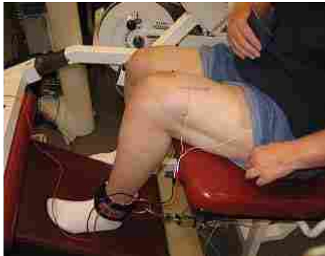
FIGURE 1. Quadriceps strength and activation testing. Strain gauge is attached to seat frame and to subject's ankle at 90° to leg. Knee flexed to 75°. Two electrodes were placed over the vastus medialis and proximal rectus femoris of the quadriceps.
